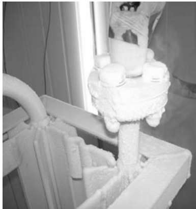
(a) Frost type near inlet of the vaporizer (porous frost type)
